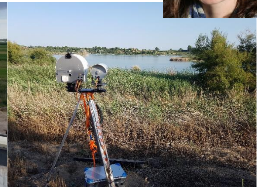
Landscape scale H + L_p E with combined Optical and Microwave Scintillometers
