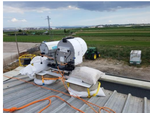
Landscape scale H + L_p E with combined Optical and Microwave Scintillometers
