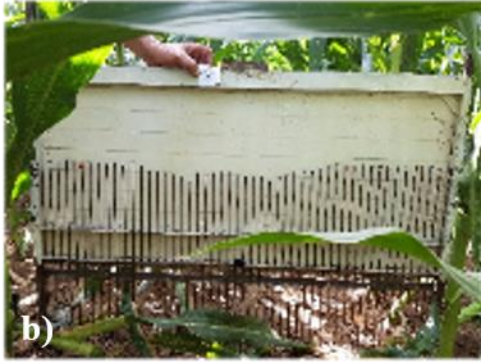
(a) soil moisture probe (b) a pin profiler picture, plot 25 (alfalfa), on July 23 (c) hemispherical photo maize.
